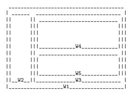
A new live window W2 is created, to the left of the internal window W3. A new internal window W1 is created, becoming the new root window.
