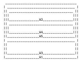
A new internal window W5 has been created; its children are W2 and the new live window W4. Now, W2 is the only sibling of W4, so enlarging W4 will try to shrink W2, leaving W3 unaffected. Observe that W5 represents a vertical combination of two windows embedded in the vertical combination W1.
