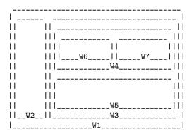
Deleting W5 in this configuration normally causes the deletion of W3 and W4. The remaining live windows W2, W6 and W7 are recombined to form a new horizontal combination with parent W1.
