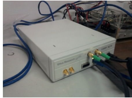
Figure 8. USRP N210 for software-defined FMCW radar system prototyping
