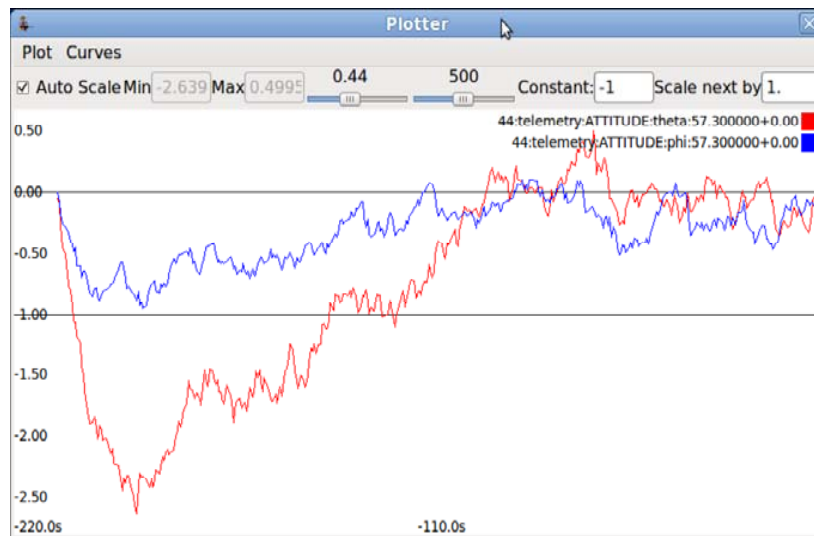
Stabilization of rolls and pitch angle after power up
